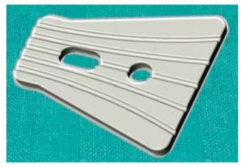
**Fig. 1:** Esnoper<sup>®</sup> trapezoidal design with longitudinal irrigation channels, a round hole for scleral fixation and a larger hole to improve the aqueous humor flow
