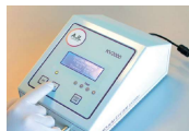
17. To deactivate the vacuum system or turn off the pump, keep pressing the pedal or the OFF button
