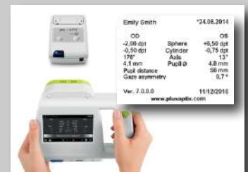
Label printing with plusoptiX A12R
